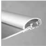
Profile / UYUP002100 1" Aluminium Security profile set (top & bottom) in 118.11" without springs. Top Profile is silver anodized. Bottom profile is mill finished.
